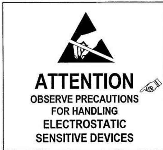
FIGURE 2: SENSITIVE ELECTRONIC DEVICE (TYPICAL EXAMPLE) CAUTION LABEL
