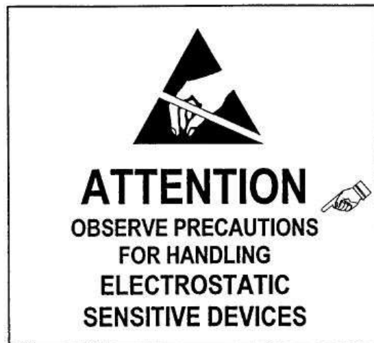
FIGURE 2: SENSITIVE ELECTRONIC DEVICE (TYPICAL EXAMPLE) CAUTION LABEL
